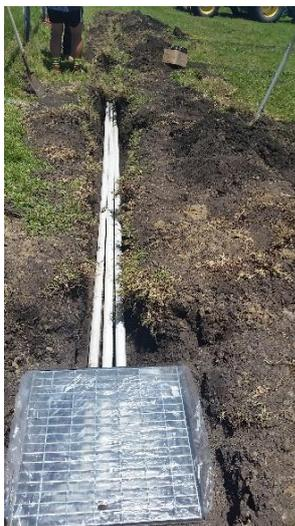
Outflow from each treatment trench was combined, and measured by flow gauges.
