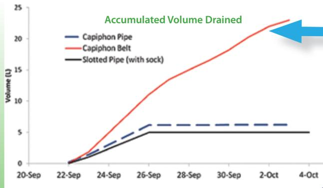
Capiphon™ pipe acts much sooner than slotted pipe to rid ground of excess water
